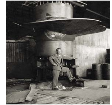
One of the three Kaplan turbines. Mr John Woodman 's personal photo collection.
